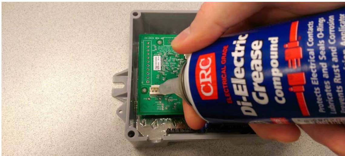
Figure A - 3. Apply the Compound to the GPR2-PT Pulse Input Connector
