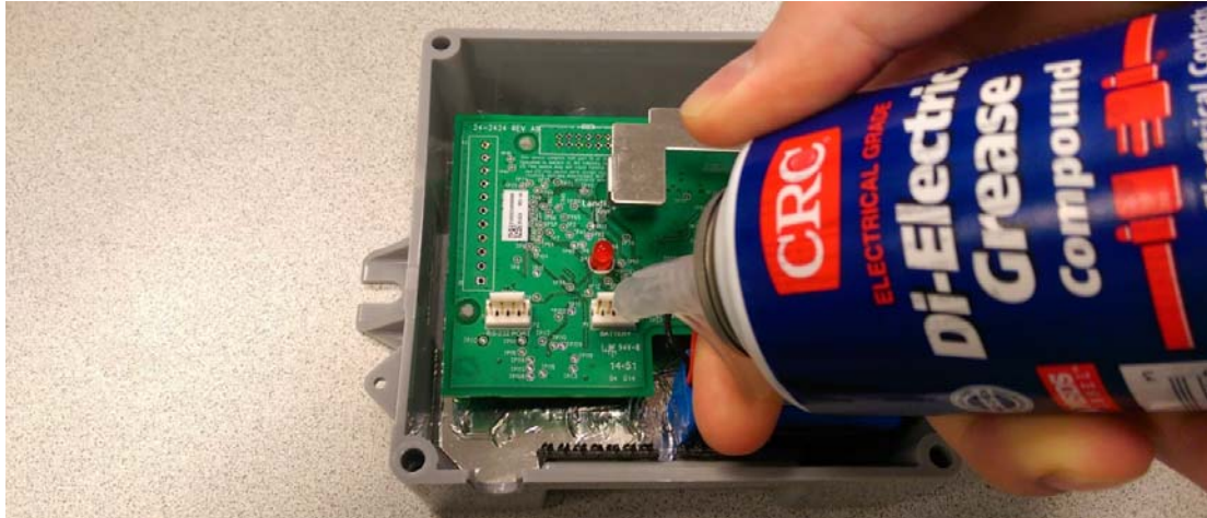
Figure A - 2. Apply the Compound to the Battery Connector
