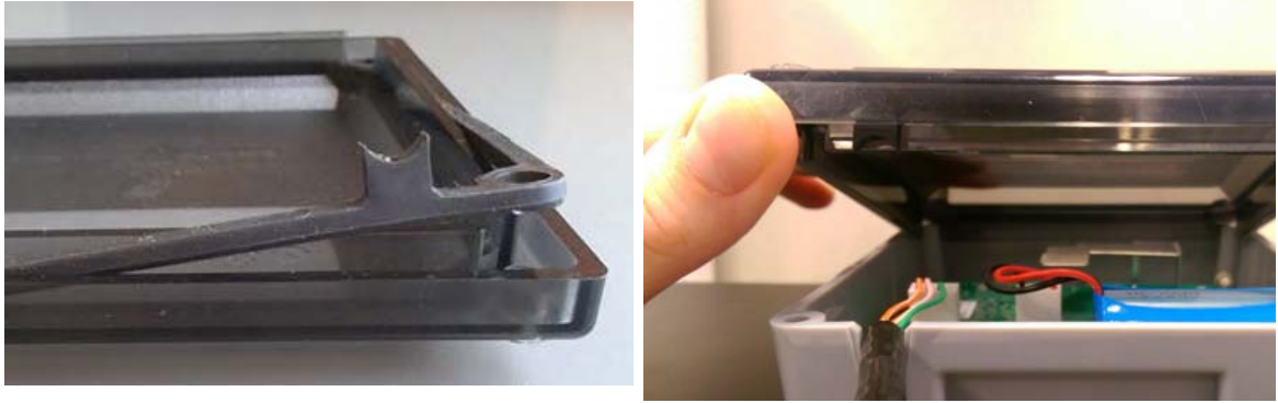
Figure 2 - 22. GPR2-PT Cover Gasket Tab and Cover Strain Relief Slot
