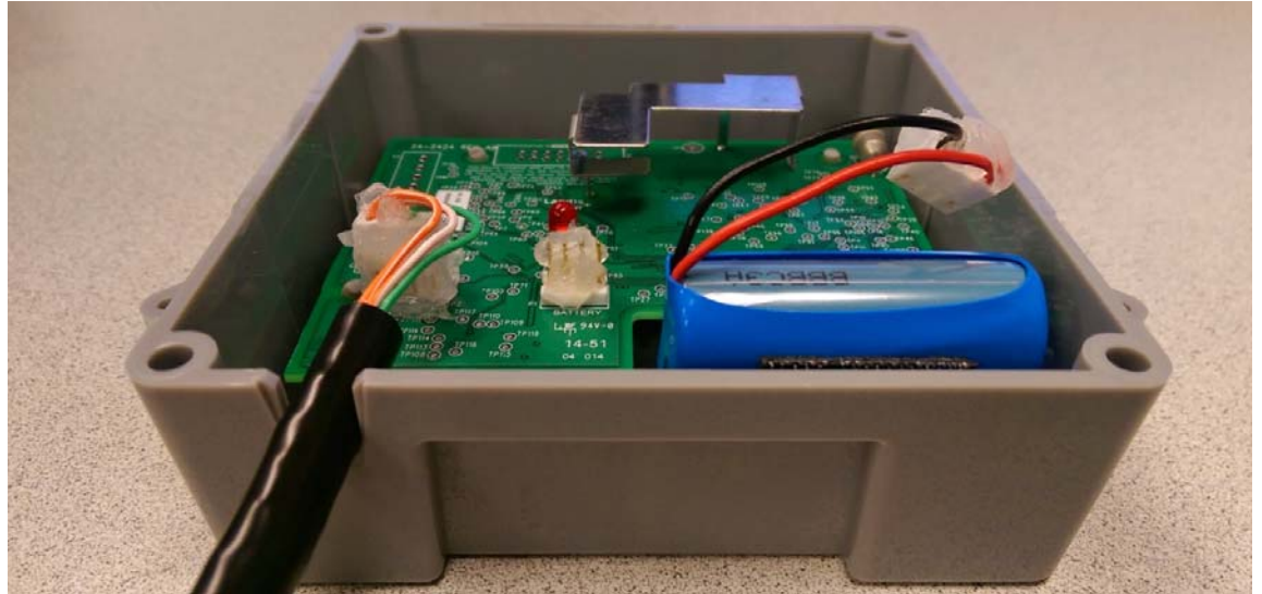
Figure A - 8. GPR2-PT Serial Cable Pressed Into Strain Relief Slot
