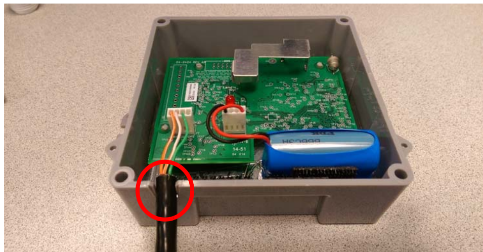
Figure 2 - 21. Serial Cable Must Route Through GPR2-PT Strain Relief Slot
