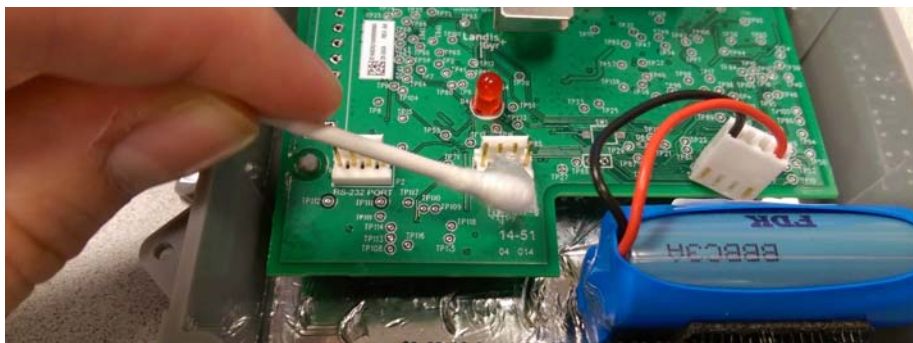
Figure A - 4. Force the Compound between Connector Pins
