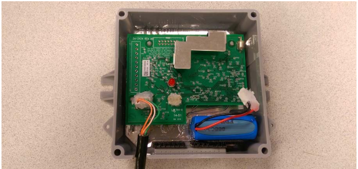
Figure A - 7. Arrange Cables As Shown Before Installing the GPR2-PT Cover
