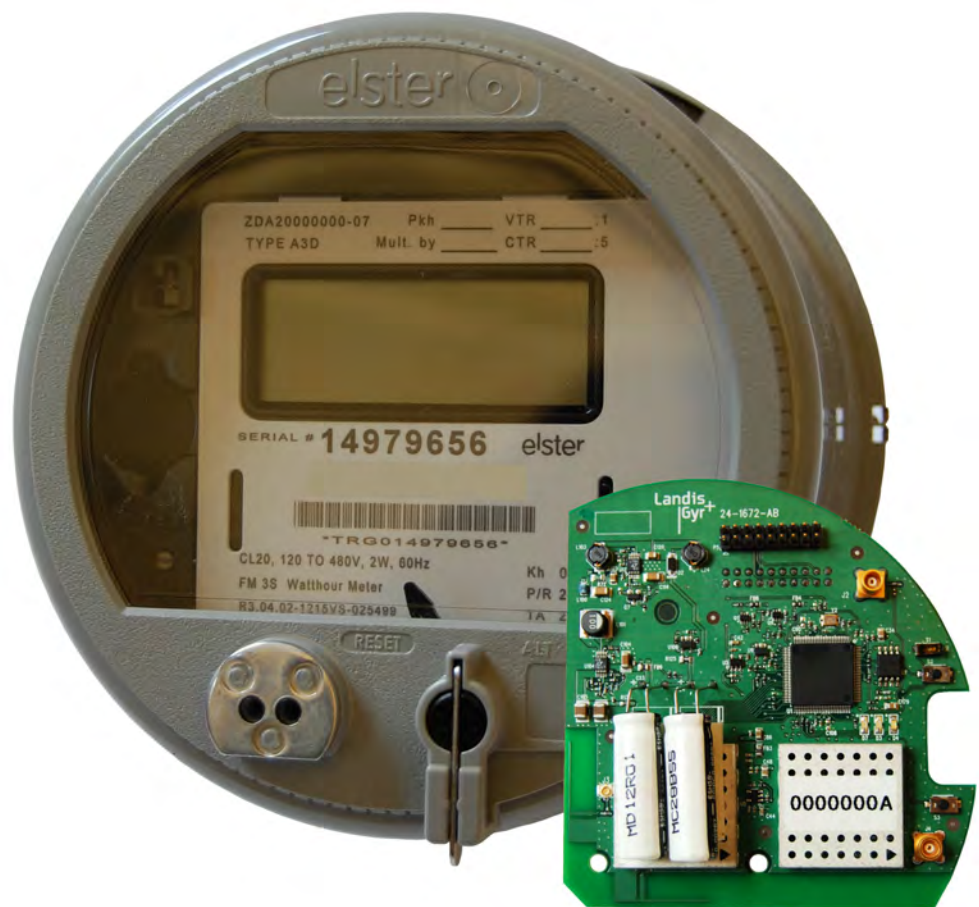
Figure 1 - 1. Gridstream RF Enhanced Elster A3 Meter and Module
