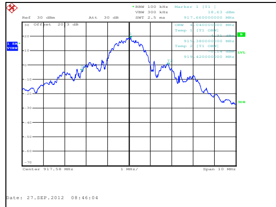
Figure 7.3.2-2: 99% Bandwidth Plot – Port B
