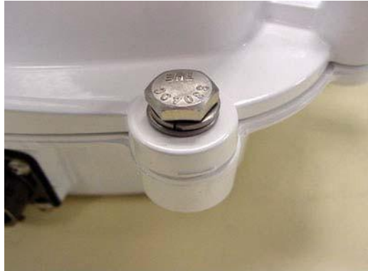
Figure 5 - 2. RF Filter retrofit unbolt lid and base
