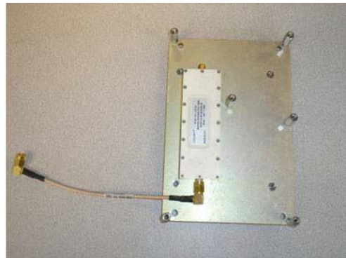
Figure 5 - 7. Installing RF Filter
