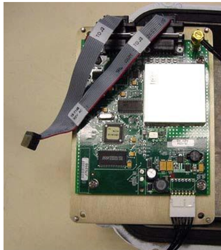
Figure 5 - 5. RF Filter retrofit remove UtiliNet S3 PCBA
