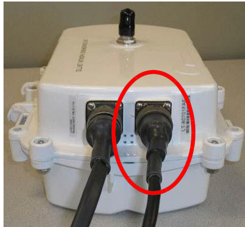
Figure 3 - 4. Concentrator with programming cable
