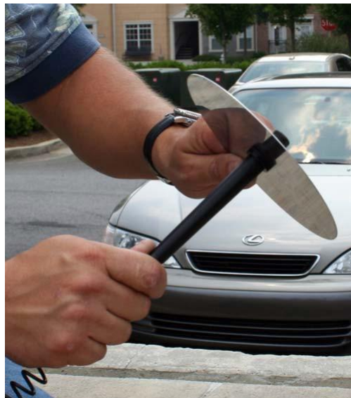
Figure 4 - 8. Putting ground plane on antennas
