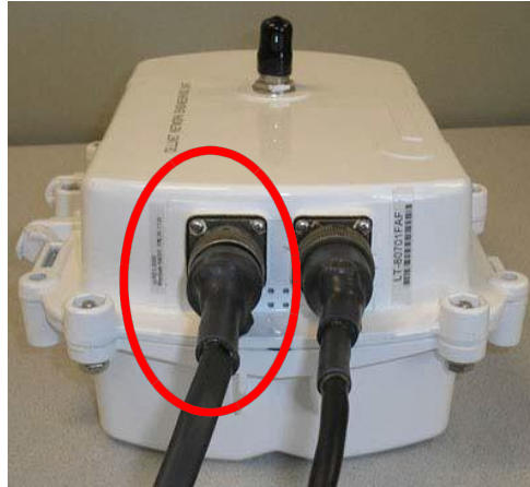
Figure 3 - 1. Concentrator with programming cable
