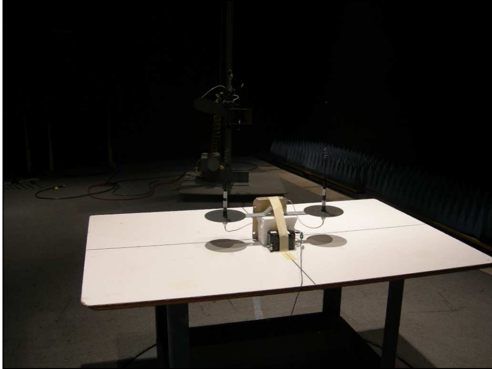
Figure 6: Radiated Emissions – ZPOS
