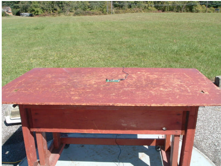
Pictorial 1 R7H-BKLINK-R Radiated Emissions Test Set-up
