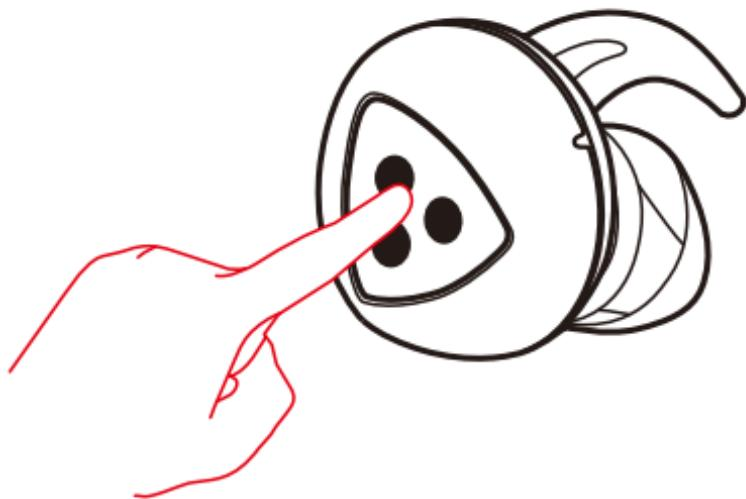
Press and hold the entity button for 2 seconds when power is off
