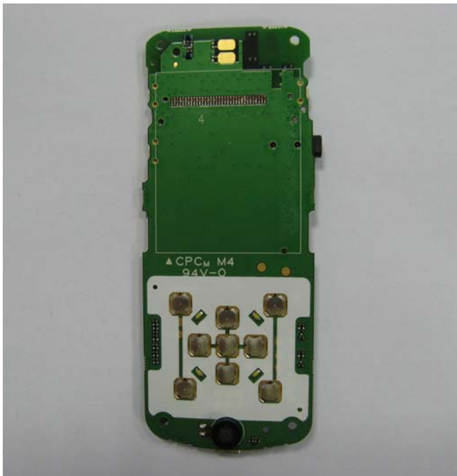
Picture 2: Front view of PCB with the screen removed
