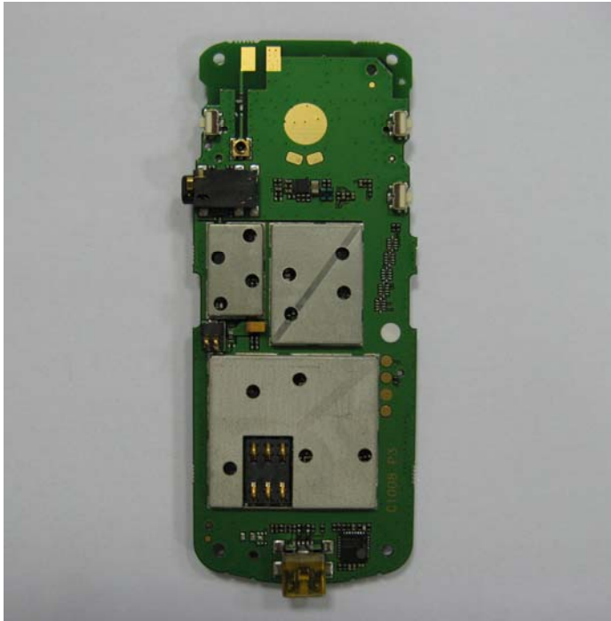
Picture 4: Back view of PCB with antenna removed
