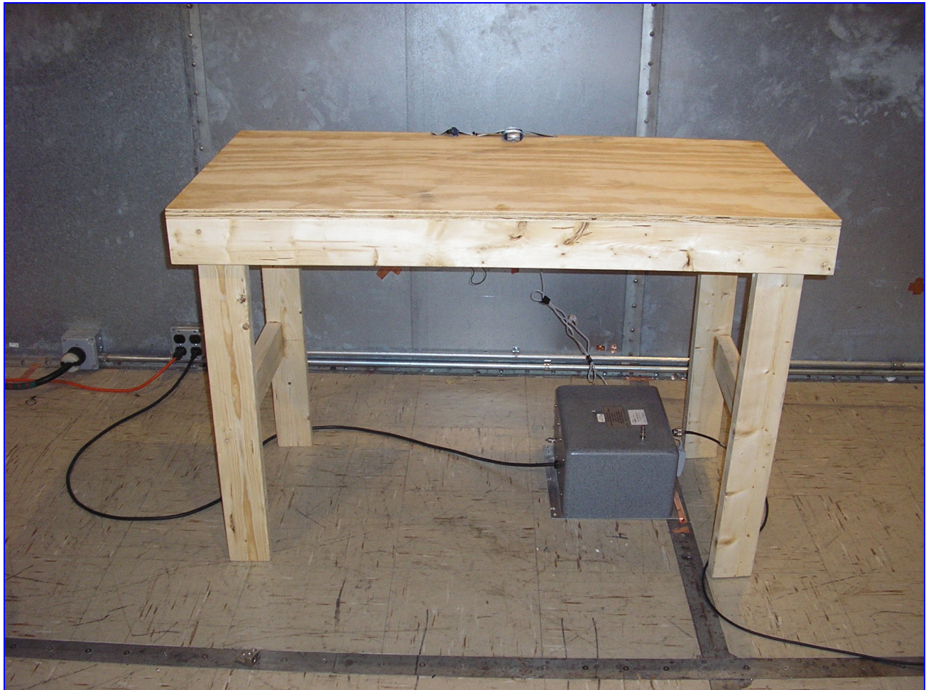
Photograph 1. Conducted Emissions Test Setup
