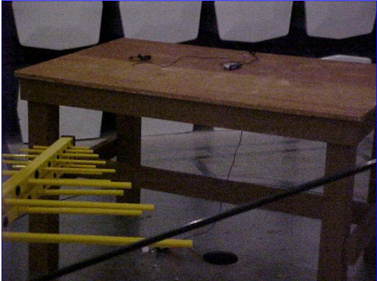
Photograph 2. Radiated Emission Limits Test Setup
