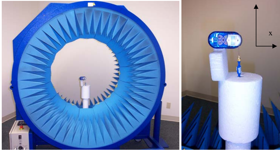
Figure 2: Test of phone in Anechoic Chamber.
