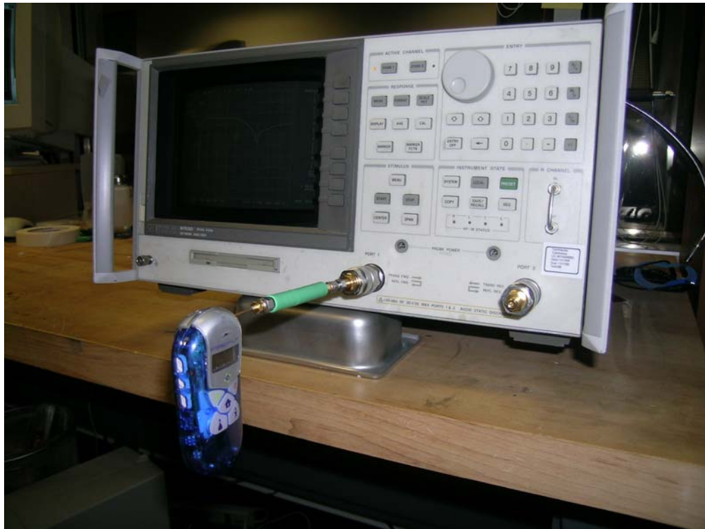
Figure 1: Test of Antenna in Phone.
