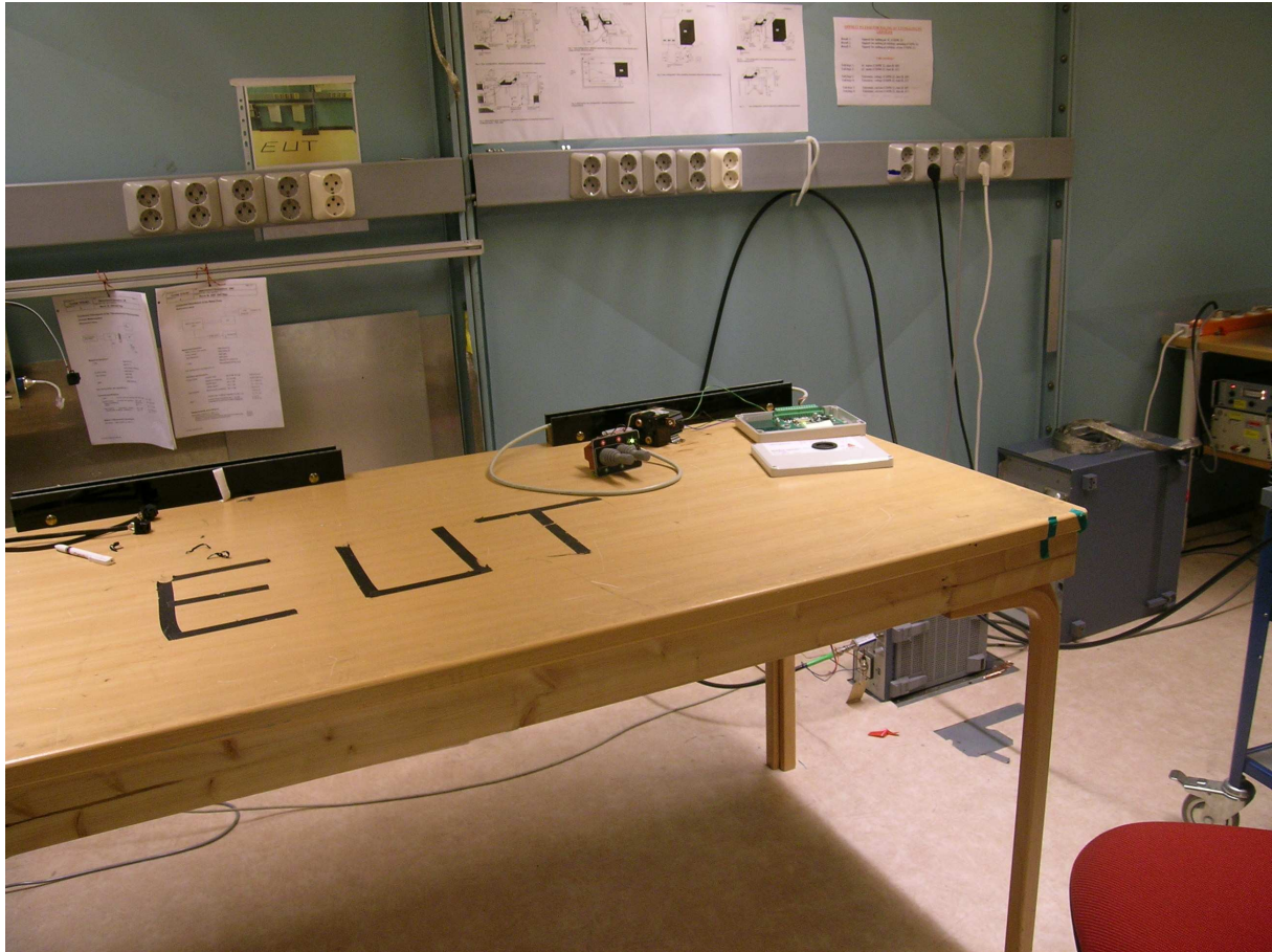
ECU-01 – Conducted emission test set-up
