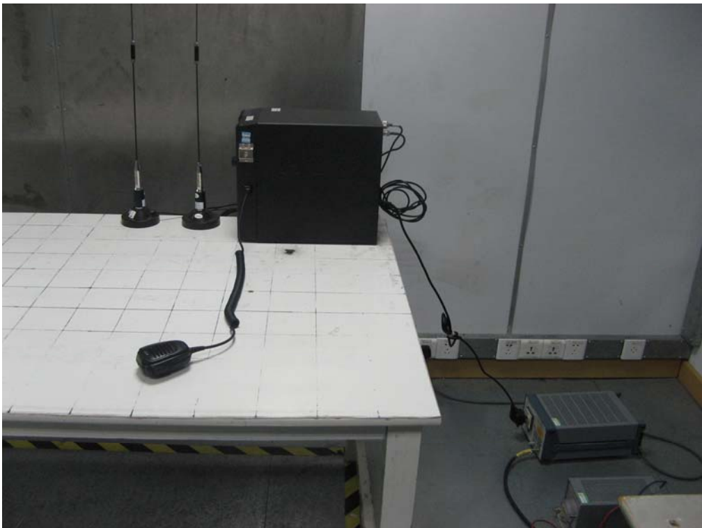
CONDUCTED EMISSION TEST SETUP
