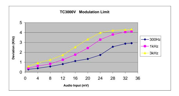
For 12.5KHz Channel Spacing:
