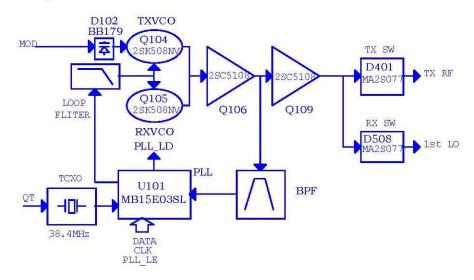
PLL circuit mainly generates RF carrier signal (for Tx) and 1<sup>st</sup> local oscillator (for Rx).
