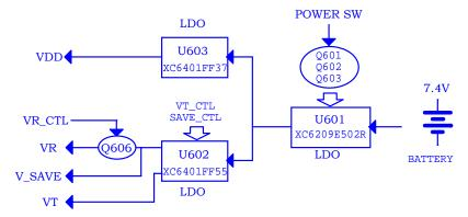
Power Supply: After a 7.4V battery voltage goes through LDO IC U601, a steady 5V DC voltage is generated. Then, the voltage is divided into 2 ways. In one way, a 4.5V DC voltage that supplying power to Tx, Rx and VCO circuit is generated after it is converted at LDO U602. In the other way, a 3.3V voltage that supplying power to MCU, EEPROM and PLL is generated after it is converted at LDO U603.
