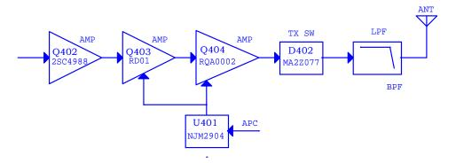
The carrier signal having been modulated at Q109 is power amplified at Q402. Then, the signal enters Q403 so that enough power is achieved to drive final power amplifier. At Q404, the input RF signal is power amplified again to acquire the demanded power. By then, the RF signal goes through diode D402 and enters a low pass filter (LPF) circuit. In LPF, the higher harmonic is filtered. At last, the signal is transmitted from the antenna.
