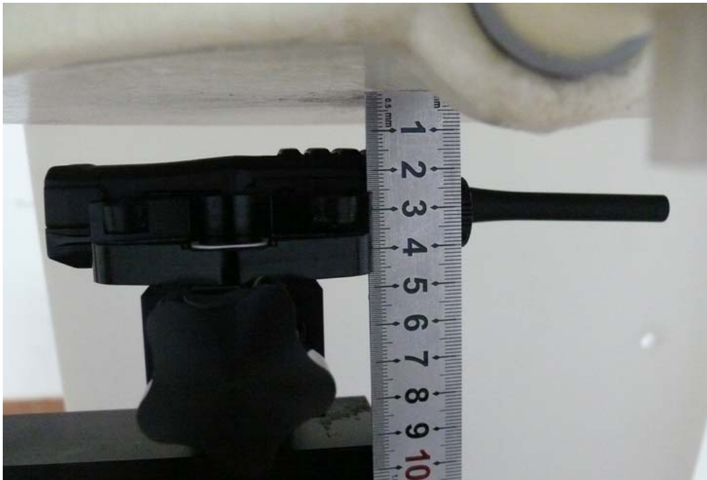
Picture 4: Face-held, The EUT display towards phantom, the distance from EUT to the bottom of the Phantom is 15mm
