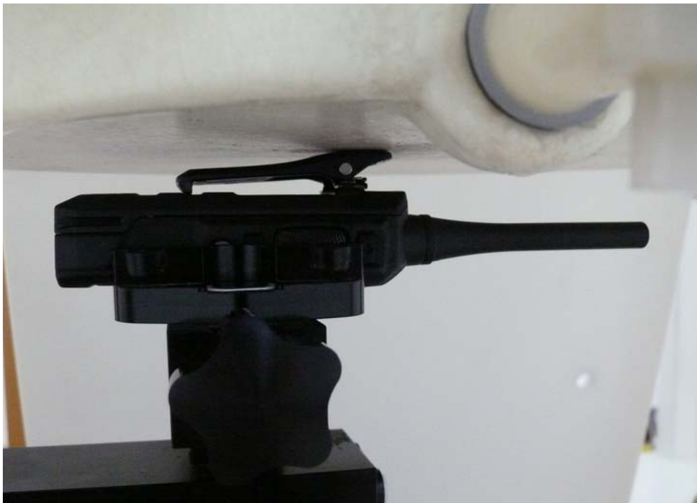
Picture 5: Body-worn, The EUT display towards ground, Belt clip attach the Panntom
