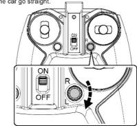
. If the remote control car turns left while moving forward 12. If the remote control car turns right while moving forward without touching the right control lever, twist the fine-tuning knob of the remote control anticlockwise until the car go
