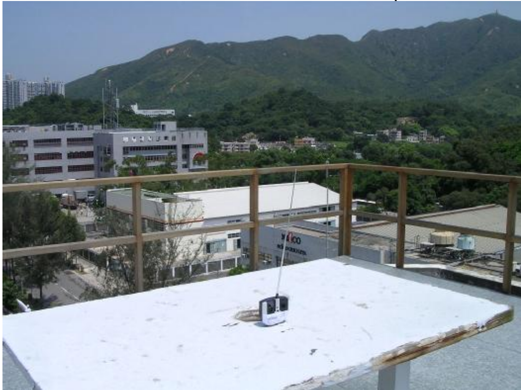
Measurement of Radiated Emission Test Set Up
