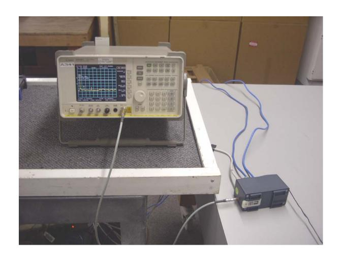
Conducted Emissions at Antenna Terminal Setup
