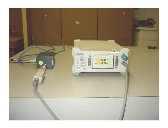
Maximum Peak Output Power Measurement Setup
