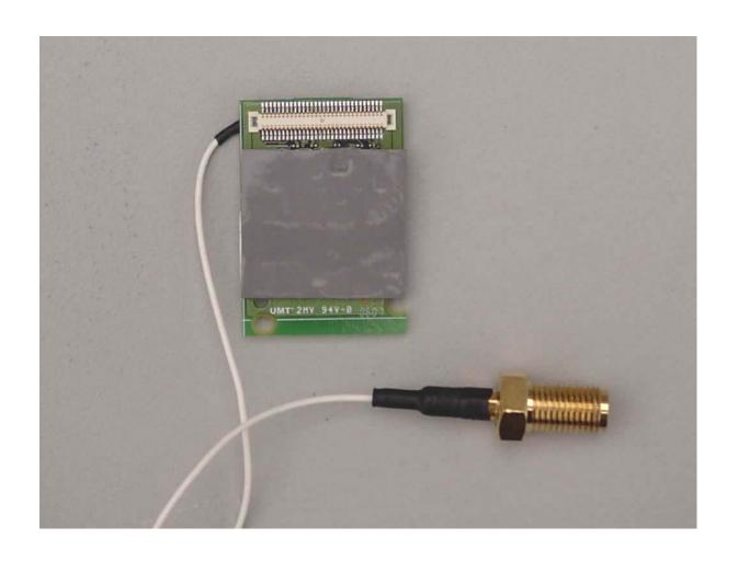
Bottom View "Transmitter Board With Insulation"
