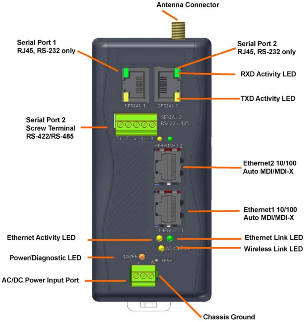
Figure 4-6. XPress DR+W Front Panel Layout
