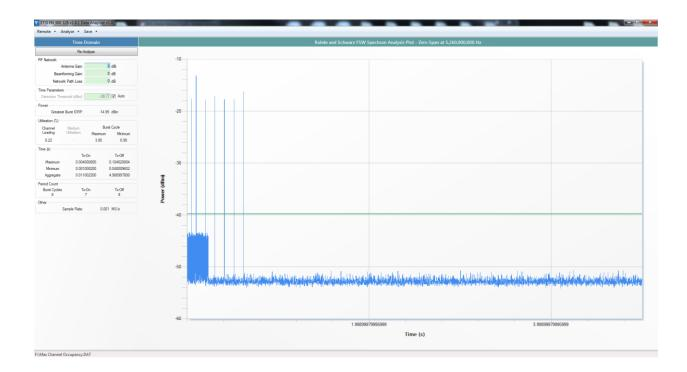
Channel Closing Time of 11 ms, trace data analyzed for aggregate TX on time (<200 ms, EUT complies)
