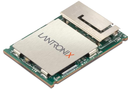
XPC2402 – LGA, On-Module Antenna
