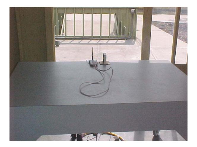
Radiated Emissions Measurement (Front View) Setup
