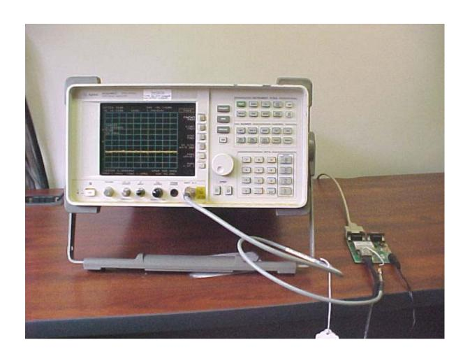
Conducted Emissions at Antenna Terminal Setup
