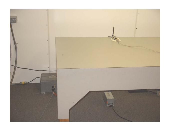
AC Conducted Emissions Measurement (Front View) Setup
