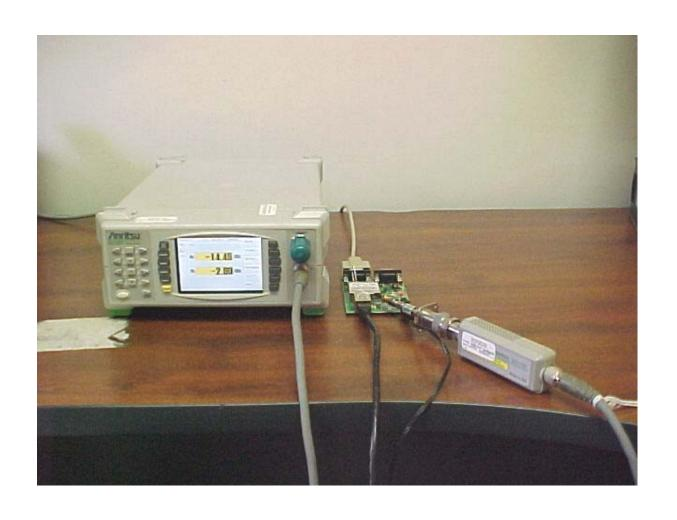
Maximum Peak Output Power Measurement Setup
