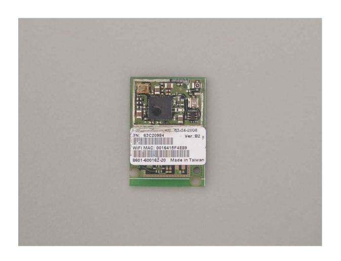
Top View "Transmitter Board, Shield Removed"
