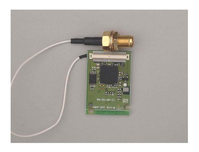
Bottom View "Transmitter Board Without Insulation"
