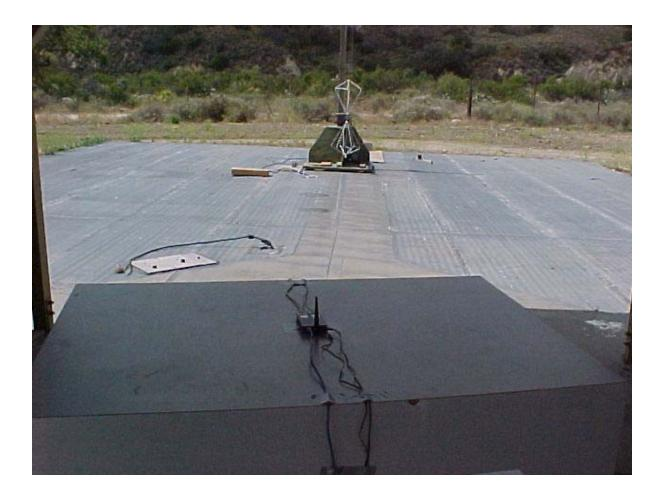
Radiated Emissions Measurement (30-100 MHz) (Rear View) Setup
