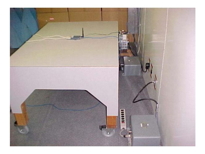
AC Conducted Emissions Measurement (Rear View) Setup
