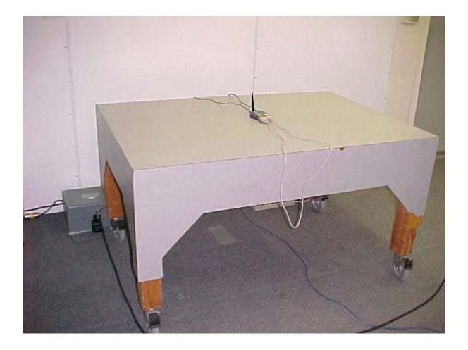
AC Conducted Emissions Measurement (Front View) Setup
