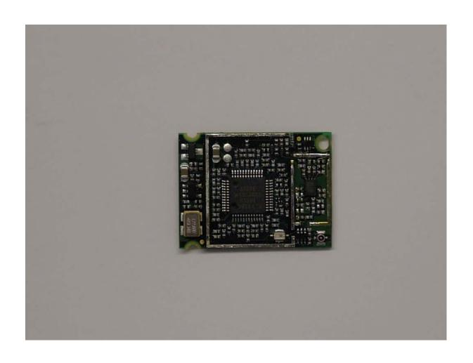
Top View "Transmitter Board, Shield Removed"
