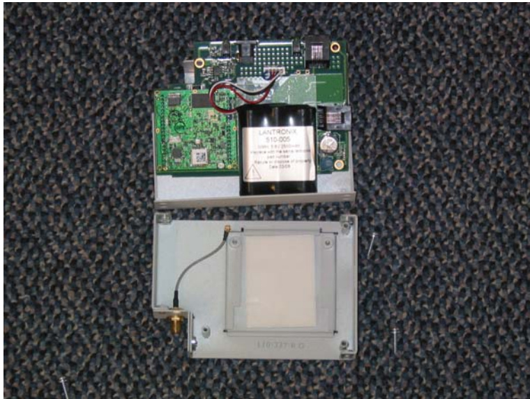
PCB on Battery Side
