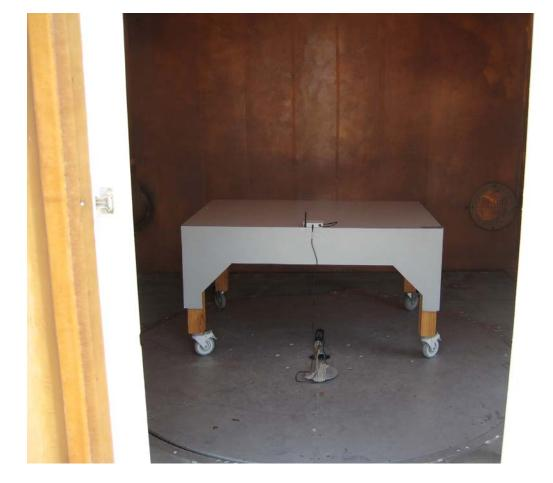
Radiated Emissions Measurement (Rear View) Setup
