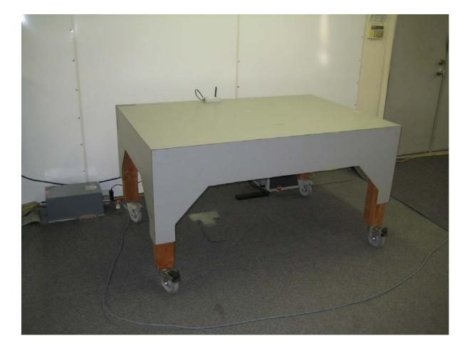
AC Conducted Emissions Measurement (Front View) Setup
