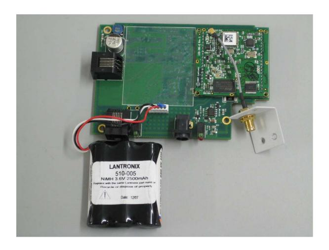
Top View of Circuit Board "Battery Removed"
