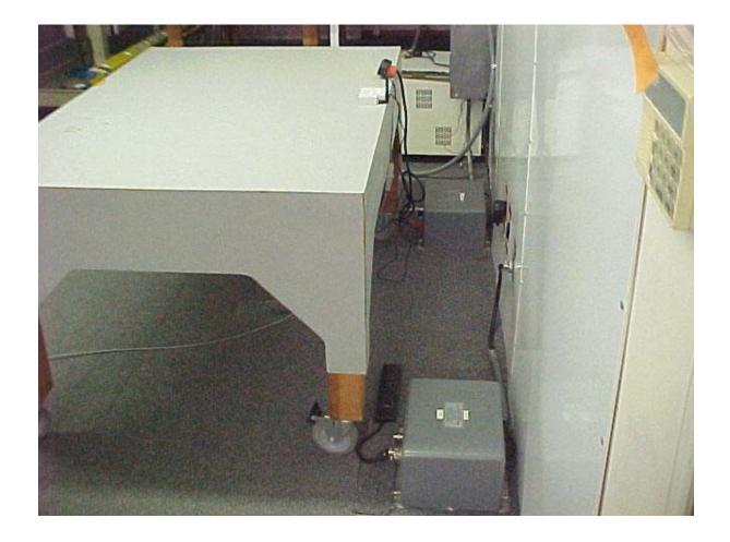
AC Conducted Emissions Measurement (Side View) Setup
