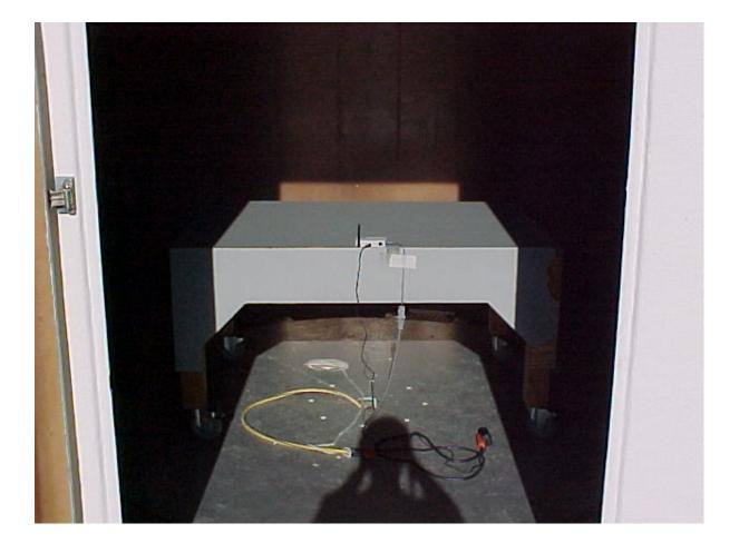
Radiated Emissions Measurement (Rear View) Setup
