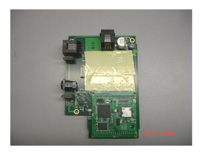
Top View of Circuit Board "Battery & Antenna Port Disconnected"
