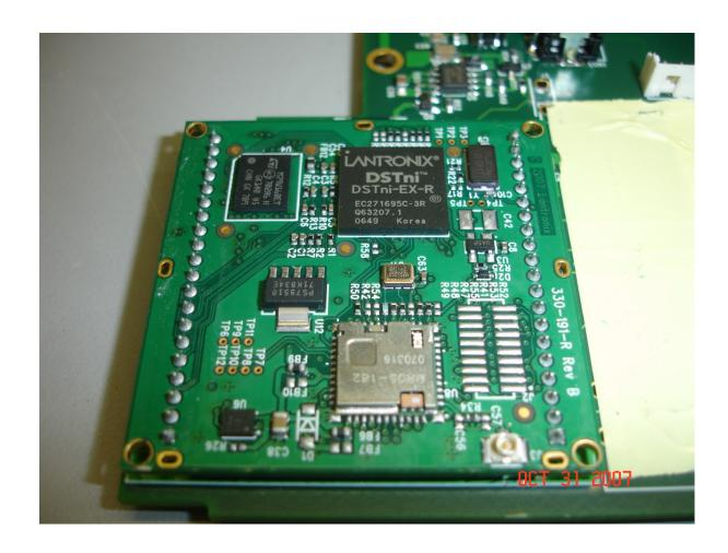
Top View "Transmitter Module Up Close
