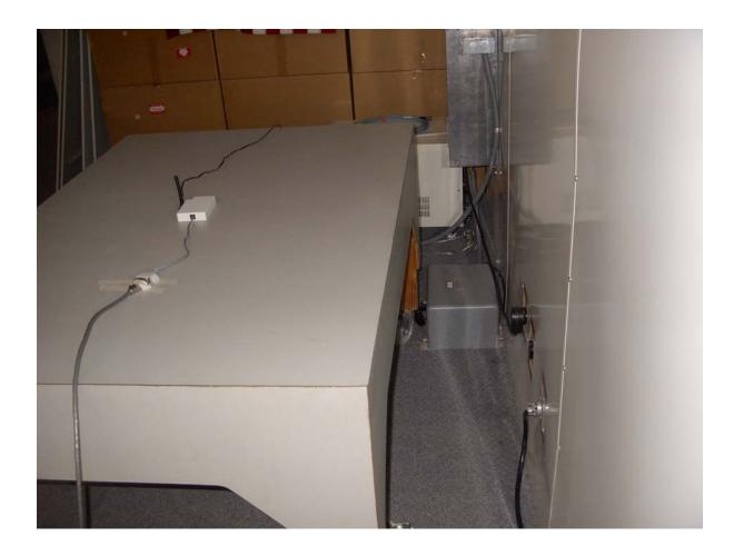
AC Conducted Emissions Measurement (Rear View) Setup
