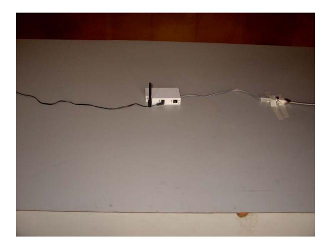
Radiated Emissions Measurement (Front View) Setup
