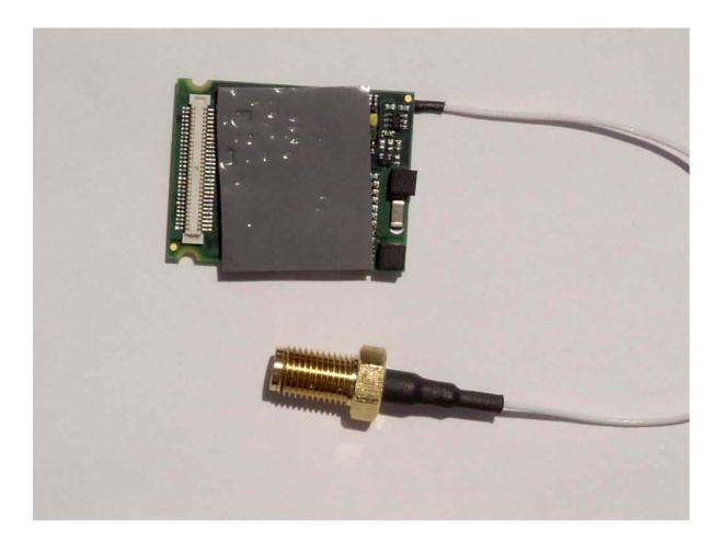
Bottom View "Transmitter Board With Insulation"
