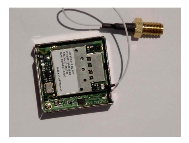
Top View "Transmitter Close-up with Top Shield Removed"
