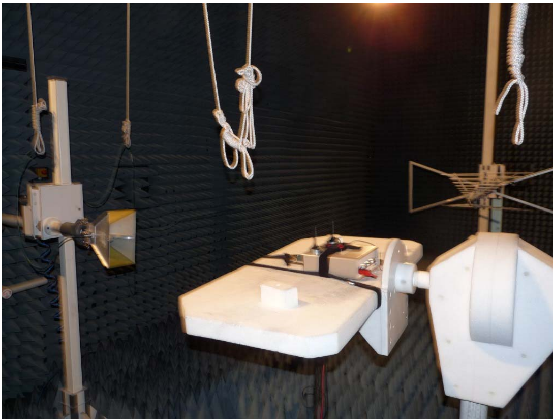
Photo 3: Test setup for radiated measurements acc. to requirements of IC (Enclosure, above 1 GHz) and acc. to requirements of FCC for intentional radiation (Enclosure, above 30 MHz)
