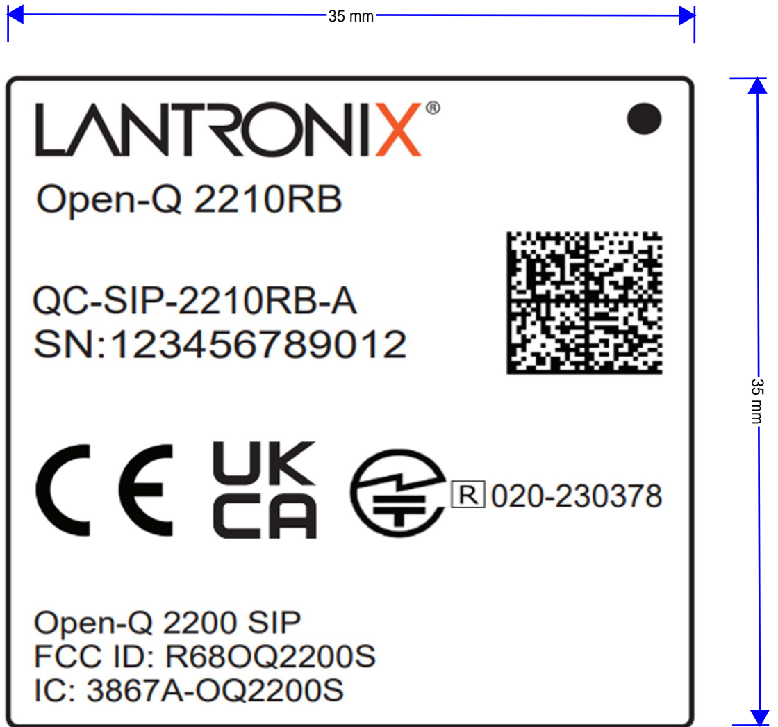
↑ Top view of Module with Label etched unto metallic shield ↑
