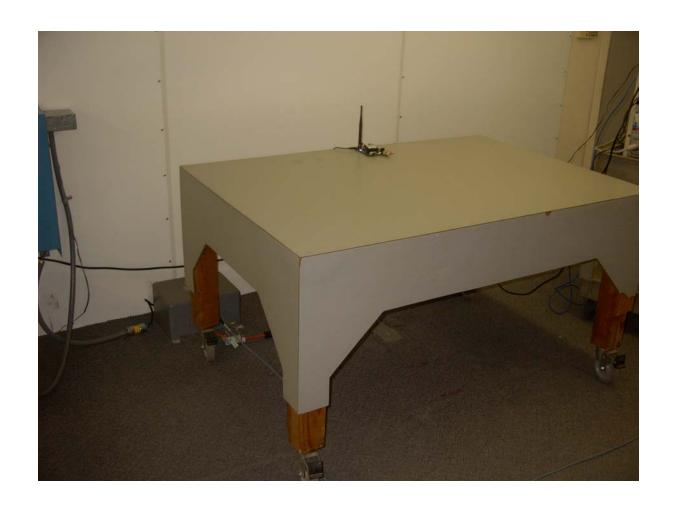
AC Conducted Emissions Measurement (Front View) Setup
