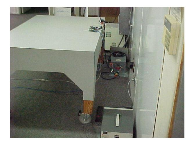
AC Conducted Emissions Measurement Setup (Side View)
