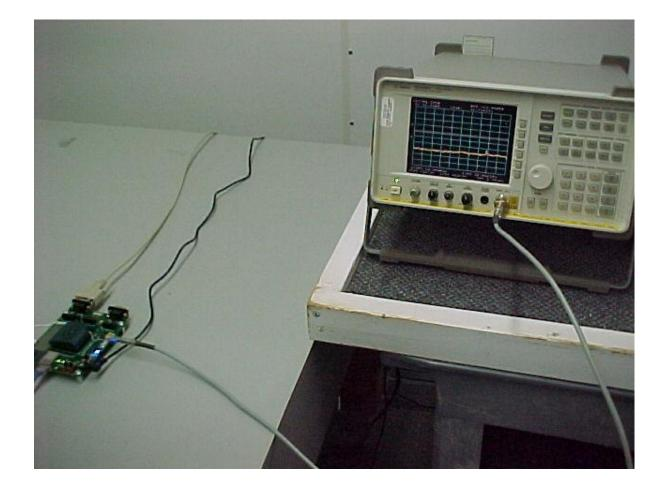
Conducted Emissions at Antenna Terminal Setup
