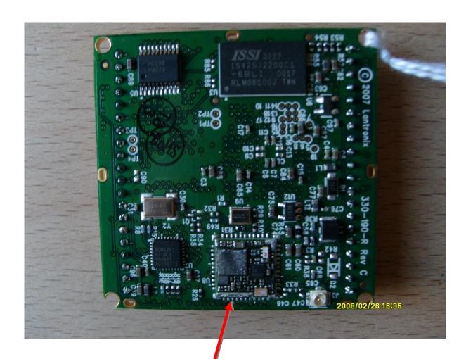
Top View – Tx Module with Shield Removed
