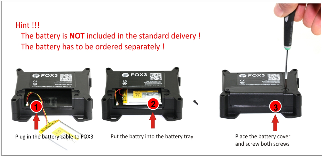
Figure 14.1: Connecting the battery to the FOX3-2G/3G/4G devices
