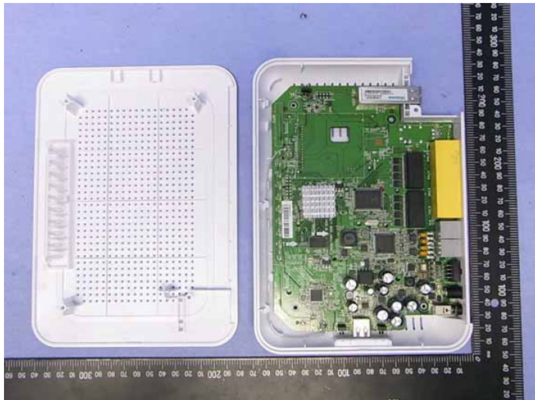
FIGURE 1 GPON SFU (M/N: 7281G) COVER REMOVED
