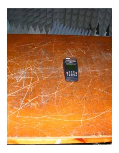
Photograph No.6 Setup for of spurious emission field strength measurements from 14 to 18 GHz
