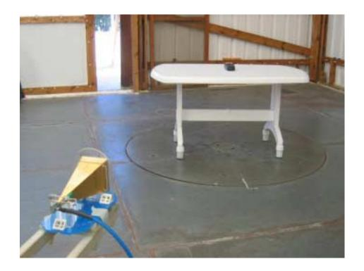
Photograph No.8 Setup for spurious emission measurements at the OATS, close view
