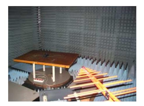
${\bf Photograph~No.5}$  Setup for spurious emission measurements in the anechoic chamber, close view
