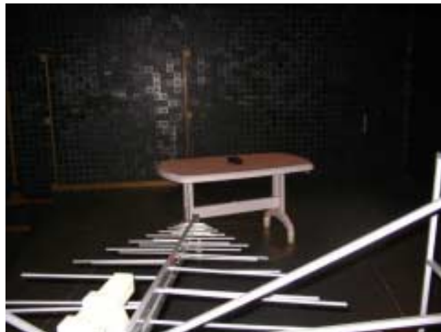
Photograph 7.2.2 Setup for spurious emission field strength measurements from 30 to 1000 MHz
