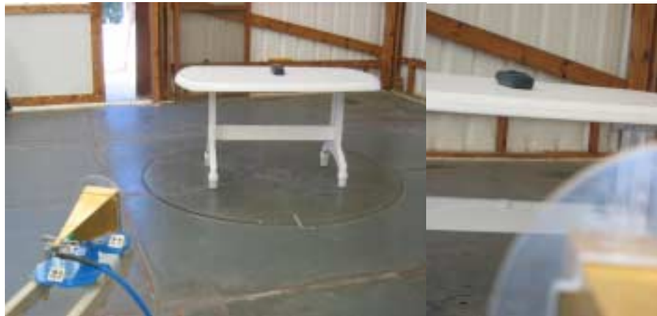
Photograph 7.2.6 Setup for spurious emission field strength measurements from 18 to 25 GHz
