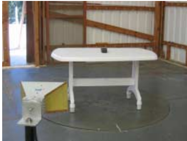
Photograph 7.2.5 Setup for spurious emission field strength measurements from 14 to 18 GHz
