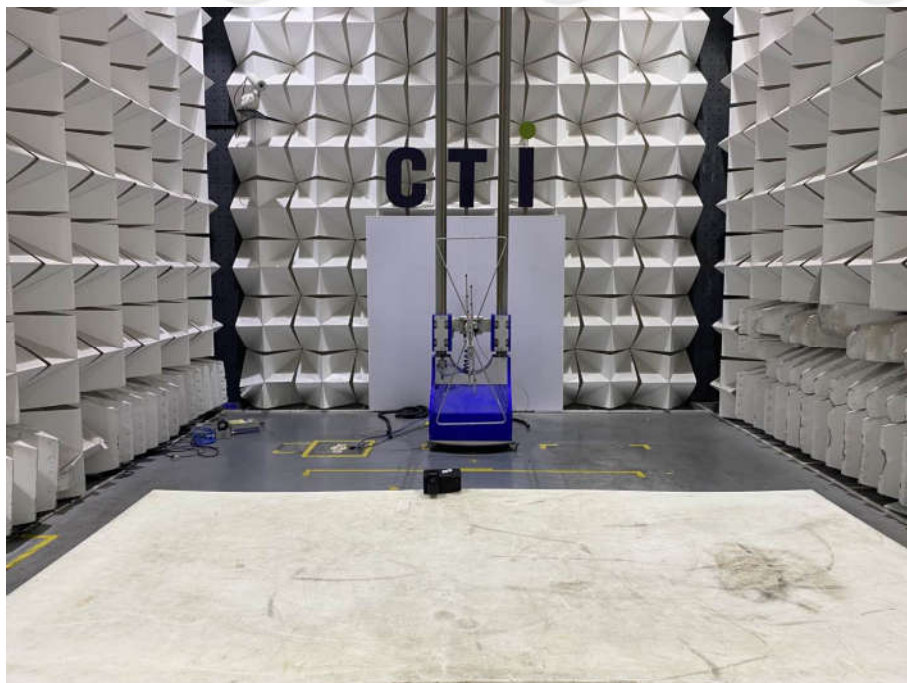
Radiated spurious emission Test Setup-1(Below 1GHz)
