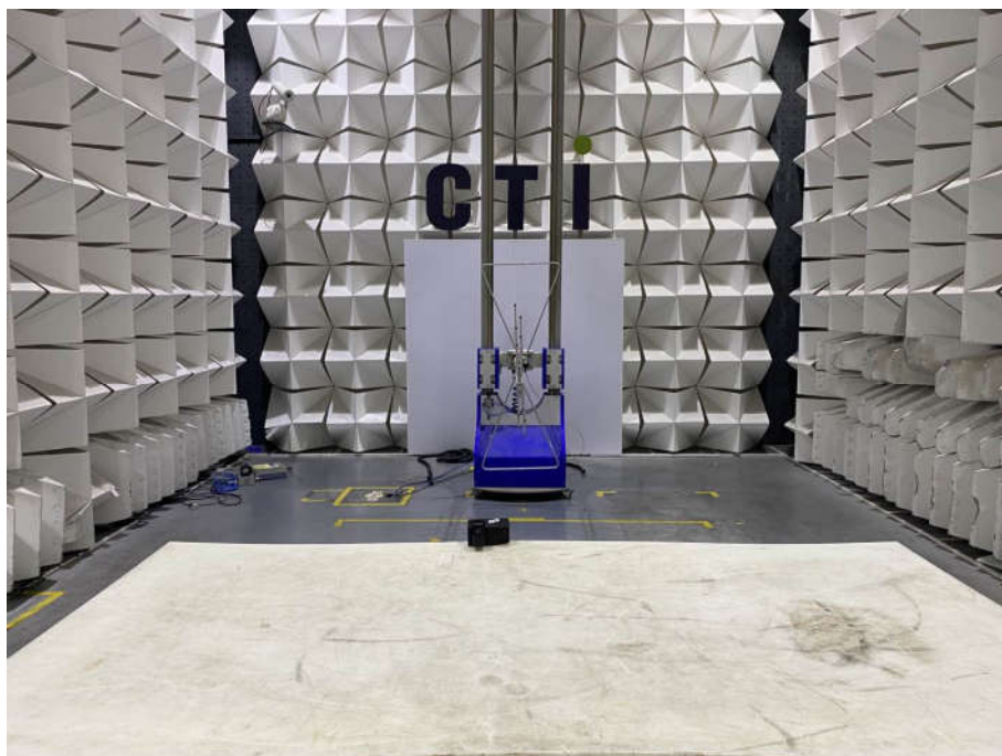
Radiated spurious emission Test Setup-1(Below 1GHz)
