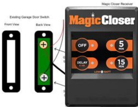
Figure 2 Connection to existing garage door switch.
