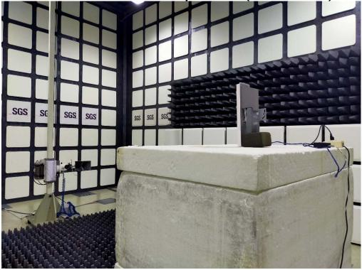
Radiated Emission Set up Photos (Front View)
