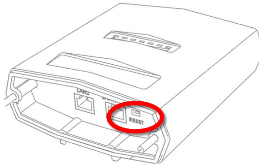
Figure 8. Cisco FM3200 Endo (Hardware RESET button port)
