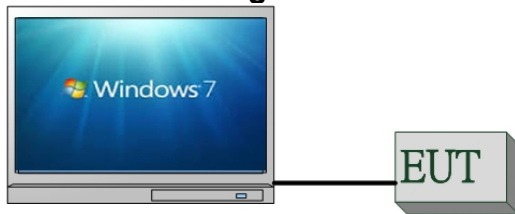
Fig. 2-2 Conducted (Antenna Port) Emission Configuration
