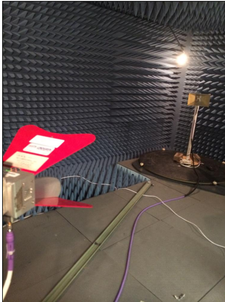
Photograph 10. DFS Calibration, Test Setup
