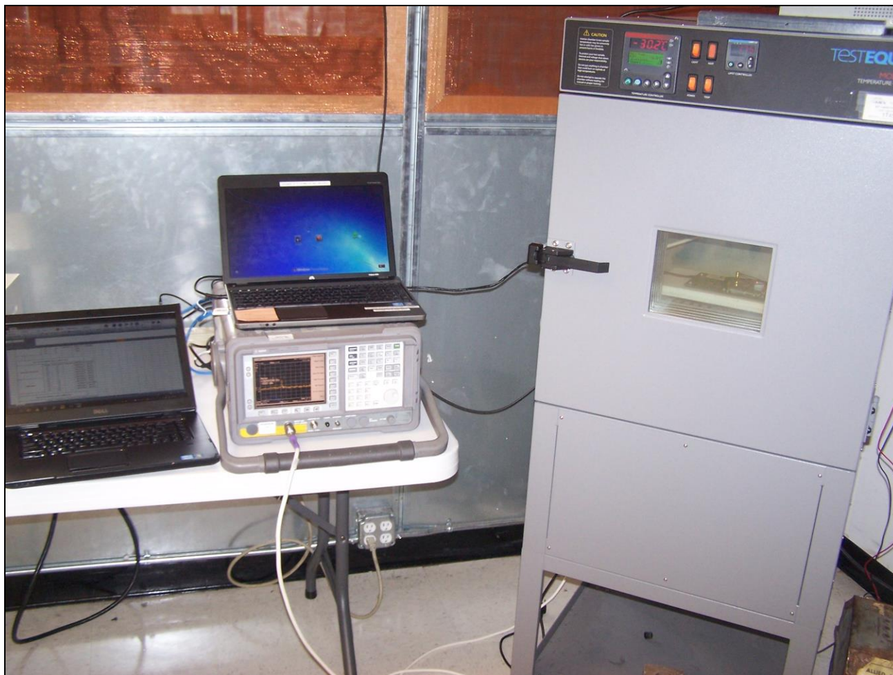
Photograph 8. Frequency Stability, Test Setup
